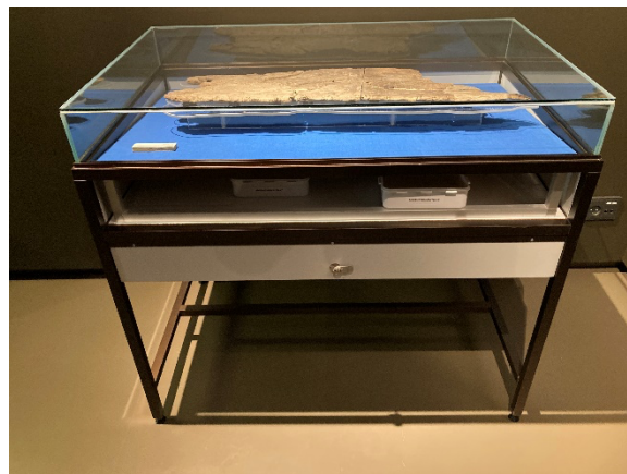
Fig 1. Relative humidity stabilisation using a saturated salt solution of magnesium nitrate in a display case containing a fragment of a PEG impregnated wooden logboat. Photo: Bevaringscenter Fyn
