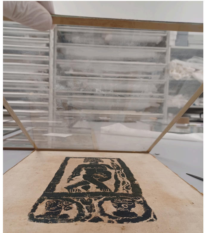
Figure 1. White deposits resulting from the chemical reaction between the textile and the glass and the creation of a microclimate
