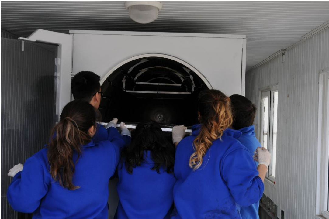
3. Putting the timbers of YK 1 in freeze dryer
