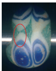
Figure 1. Glass bead installed on the stainless steel rod. The ablation site is marked with a red ellipse.
