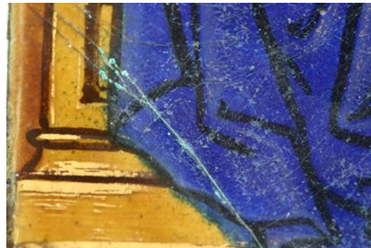
Fig. 3: Efflorescence on cracks in cover glass, lower left corner (Photo: A. Schwarz)
