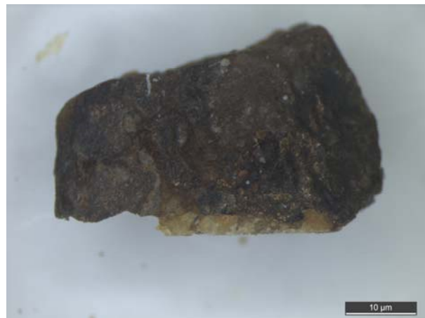
Fig. 4 – Sample taken from a star on the murals of the La Roque castle in Meyrals. View by optical microscopy (x12). On the surface, we see mainly a thick, black layer and, on the surface, gold particles.
